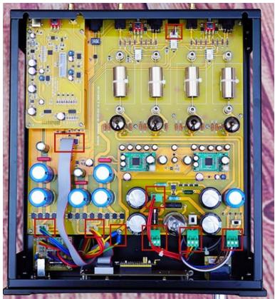
2. Remove screws, posts and unplug USB module.
