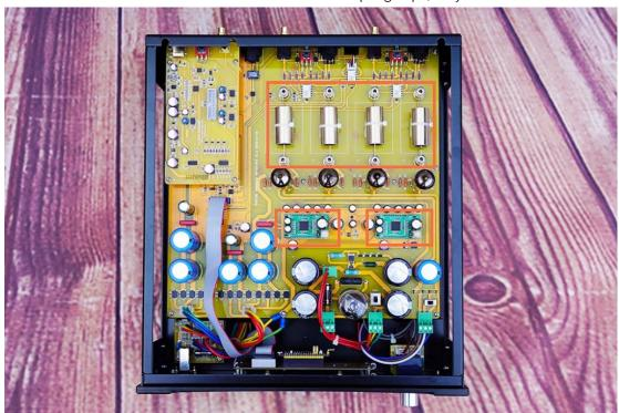
5. Install the coupling capacitors to the new motherboard. Don't touch the leads of the coupling caps, only hold their bodies. Plug in DAC modules very carefully. Please make sure the orientations of the DAC modules are correct. Also, double check, make sure all the pins go into the sockets. No any sticking out pin(s). Failing to do so can kill the DAC module(s) once powered on.
