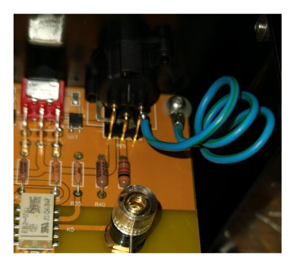
7. If you have MK1 or MK2 version of MP-D2, you also need to swap the front MCU module board to the supplied new one. MK3 users can skip this step.
