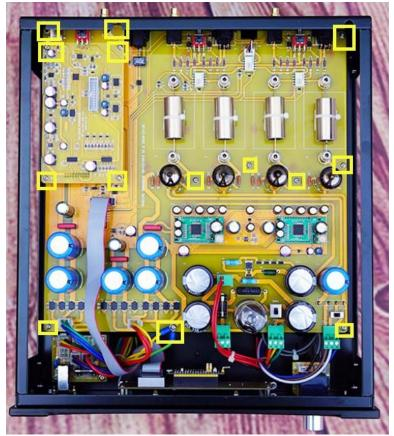
3. Remove 7 screws and gold plated RCA terminal nuts on the back.
